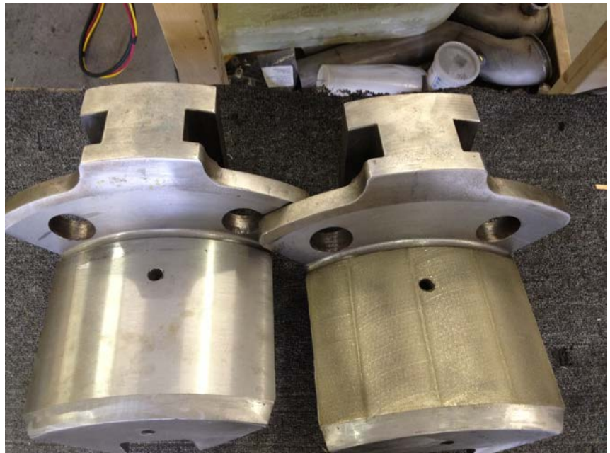
This image shows a welded and machined segment prepared for coating (left) and then a coated segment (right).
